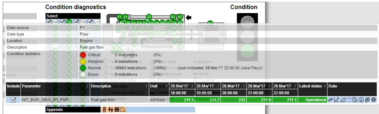
During the normal operation (when the asset condition is normal), the data sources are highlighted green. It means that the latest data that was uploaded into APM Prognostics is in the operational range. When the data starts to be in the marginal range, the diagnostic condition of asset elements (and the asset itself) becomes worse and the data sources are highlighted yellow. Finally, when the data is in the critical range, the data sources are highlighted red.
