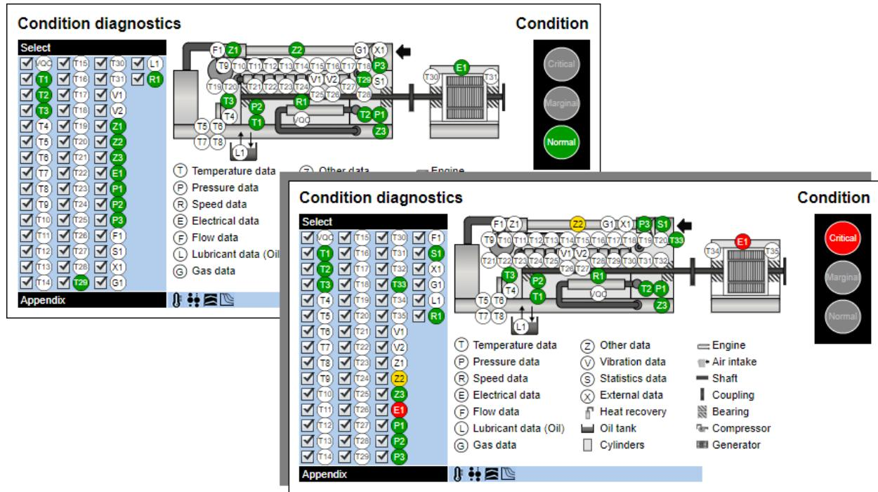
The circles on the diagram are data sources that supply information about the asset elements. The data sources usually represent measuring instruments that are on or in the asset and monitor its work and condition. The letter in the circle identifies the data source type, the numbers identify instances of a particular data source type.
