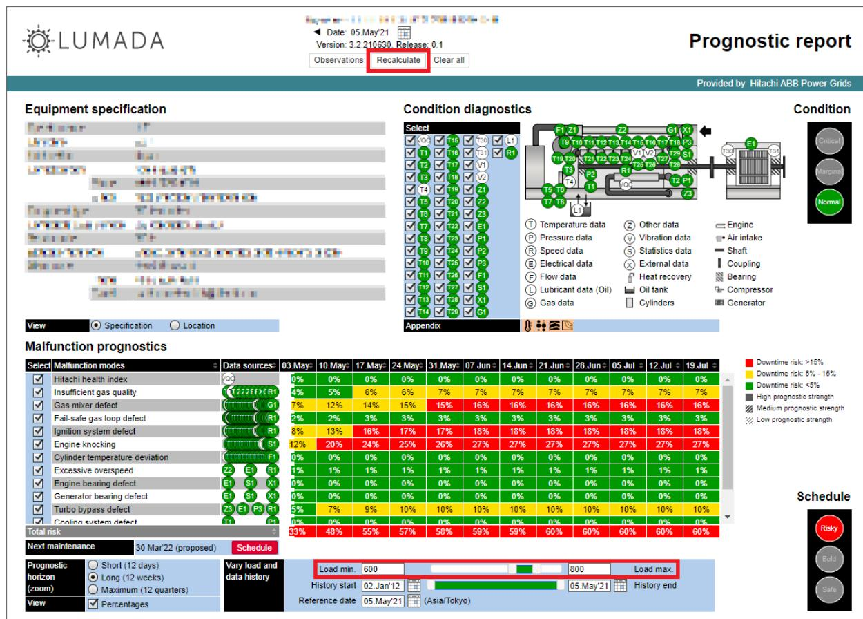
In our example, when the same gas engine asset operates within the load interval of 600 to 800 instead of 800 to 1000, the total risk of the asset becomes red on 19th July and is 15%, compared to 60% at the same date.
